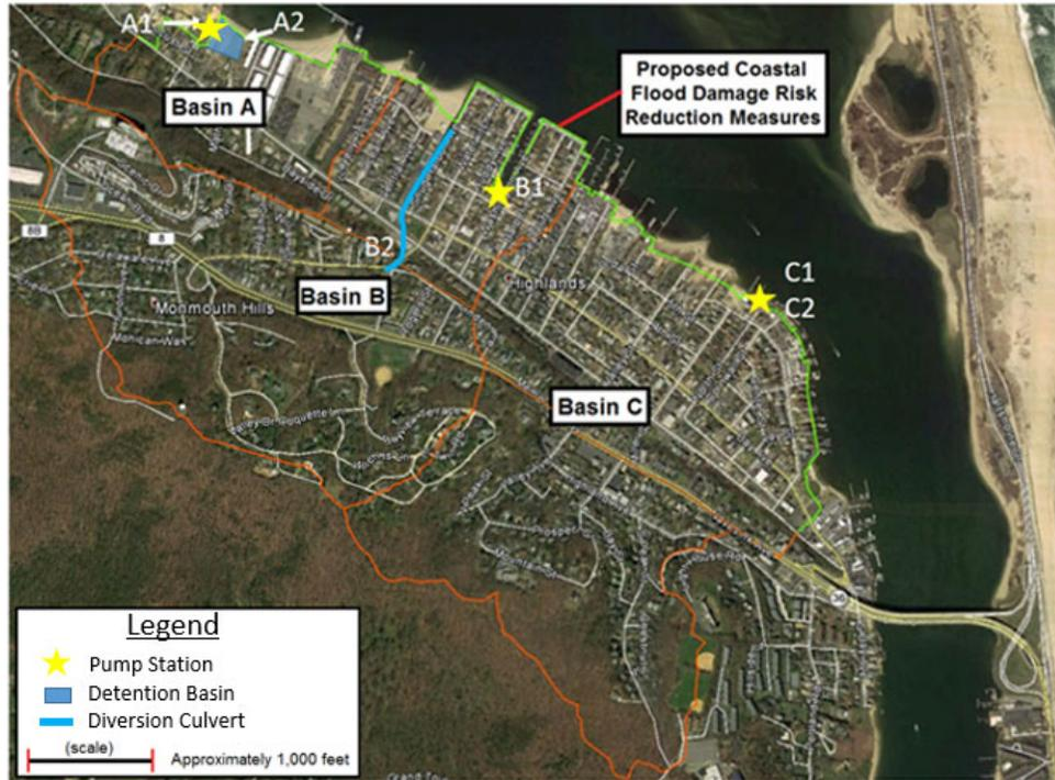
Figure B4-3: Interior Drainage Measures Proposed Alternatives
