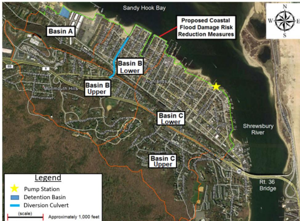
Figure B4-4: Interior Drainage Measures Selected Alternatives
